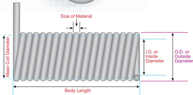
Most springs are wound with the coils touching but with minimal initial tension. For these springs the body length can be calculated by multiplying the wire diameter by the number of coils, then adding one.
