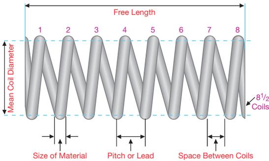
A compression spring often functions within a set amount of space or functions over a tube or rod. In these situations, this space governs the dimensional limits of the spring, controlling the allowable solid height, the inside diameter and the outside diameter. These dimensional limits, together with a spring's load and deflection requirements, determine the stress level.
